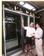
五組樣版月台幕門成功通過可靠性和耐用性測試。 Prototype platform screen doors have passed reliability and endurance tests.
